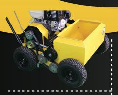
STINGER'S SUPERSEEDER 2400 IS THE MOST POWERFUL AND PRODUCTIVE POWERSEEDER IN THE INDUSTRY. THE SS2400 FEATURES COUNTER-ROTATING BLADES TO CUT THROUGH THE TOUGHEST OF SOIL CONDITIONS.
